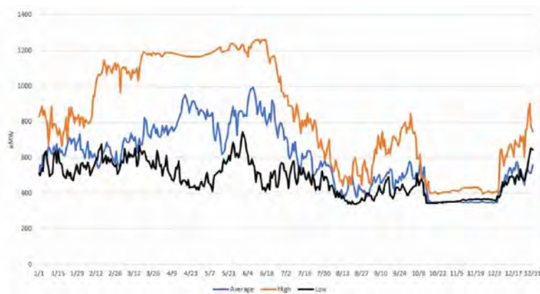
Figure 5: Daily High, Average and Low Hydro Energy Budget Profiles for Idaho Power
